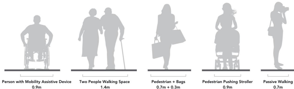
Figure 3: An illustration from Toronto's Complete Streets Guidelines showing the width requirements of different types of pedestrians ( 2017b , p. 79).
